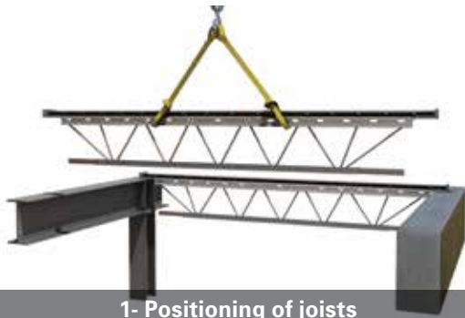
1- Positioning of joists
