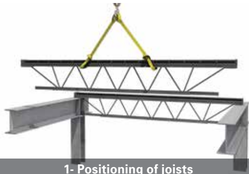
1- Positioning of joists
