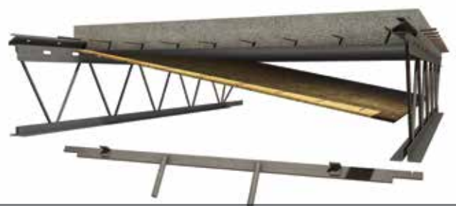
6- Removal of plywood forms
